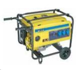
AC Rated Power ....: 4 kW AC Max. Power.....: 4,5 kW AC Voltage ...... 230 V AC Rated Current ...: 17,3 A Fuel Tank Capacity.: 25 lt. Oil Capacity..... 1,1 lt. Fuel Consumption..: 3,3 lt./hour Dimension (LxWxH).: 700 x 560 x 565 mm Weight ..... 73 kg Starting Type .....: Recoil Start Sound Level(LpA)...: 77 dB(A)@7m
