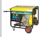
AC Rated Power ....: 6,3 kW AC Max. Power.....: 6,8 kW AC Voltage .....: 230 V AC Rated Current ...: 27 A Fuel Tank Capacity.: 16 lt. Oil Capacity...... 1,75 lt. Fuel Consumption ..: 2,8 lt./hour Dimension (LxWxH).: 720 x 500 x 770 mm Weight ...... 130 kg Starting Type .....: Electric Starter Sound Level(LpA)...: 92 dB(A)@7m
