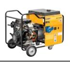
AC Rated Power ....: 8 kW AC Max. Power.....: 8,8 kW AC Voltage ...... 230 V AC Rated Current ...: 34,8 A Fuel Tank Capacity.: 16 lt. Oil Capacity...... 1,7 lt. Fuel Consumption..: 7 lt./hour Dimension (LxWxH).: 910 x 740 x 750mm Weight ..... 122 kg Starting Type .....: Electrical Start Sound Level(LpA)...: 82,6 dB(A)@7m
